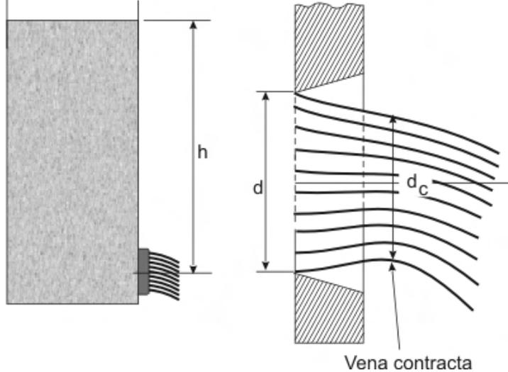
At the vena contracta, the volumetric flow rate Q of the fluid is given by
